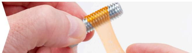
Tightly wrap and stretch VC-3 Tape around fastener 1.5 to 2 revolutions at the area of engagement
