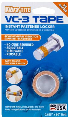
VC-3 Tape is a unique patent pending anti-vibration compound designed to prevent fastener loosening. Applied to the threads of a fastener and installed into a mating part; VC-3 Tape is ready for immediate use with no drying or curing time required. Unlike typical threadlockers, VC-3 Tape can be post assembly adjusted, removed, and re-used up to 3 times.
