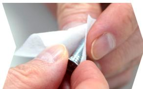
Clean fastener by removing dirt and oil
